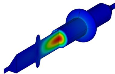
Figure 1: Electric field distribution of a  $TM_{011}$  mode trapped in the beam pipe connecting two single-cell cavities.
