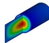
Figure 2: Electric field distribution of a  $TM_{011}$  mode of a cylindrical waveguide.
